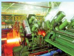
Multi-Stand pipe mill(MPM)
